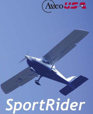
The MD-3 SportRider from FlyItalia consists of an all-metal semi-monocoque blind-riveted airframe with composite cowlings and covers. Engineered to meet the design standards of factory-produced Light Sport Aircraft regulations and the needs of the home builder too.
